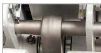
Nickel-plated suspension shaft and suspender
