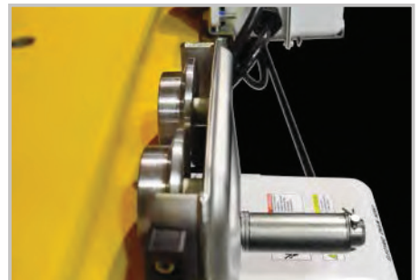
Wheels of both trolleys made of stainless steel
