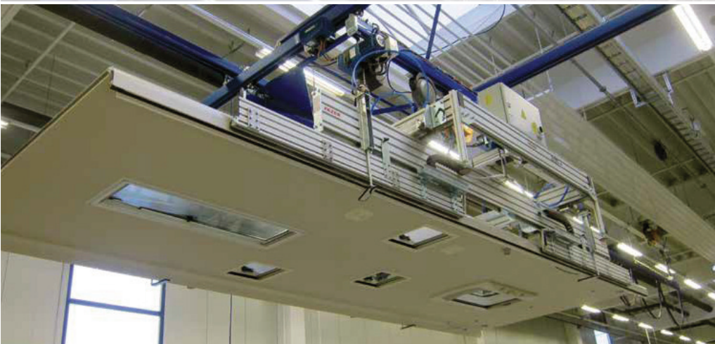
Special design for lateral engagement of camper roofs with pneumatical adjustment and mechanical undergrippers
