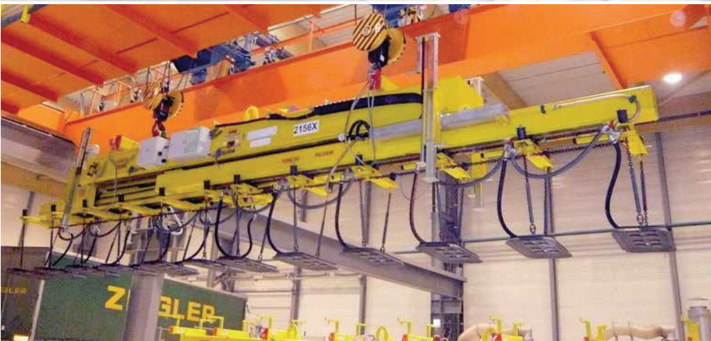
VacuGiant with 12.000 kg carrying capacity and electrically extendable main beam from 8 to 12 m
