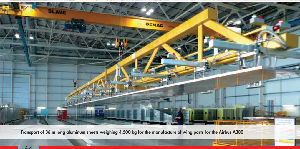
VacuGiant with 12.000 kg carrying capacity and electrically extendable main beam from 8 to 12 m
