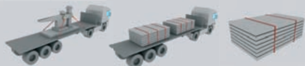
▶ Oblique fastening or in diagonal ▶ Fastening on plate ▶ Hooping
