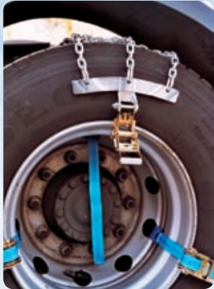
1 Place the chain on the upper part of the tire, ratchet outside, webbing inside.
