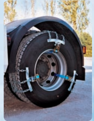
4 Strain the chain (To maximize the efficiency and reliability, we recommend to strain a second time after having driven few meters). Up to 4 units can be installed on the same tire.
