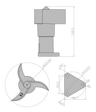
The anemometer consists of a plastic rotor impactresistant and to UV rays, at low temperatures and hail. Rotating on ball bearings, drives a magnetic contact, generating 4 pulses per revolution.
