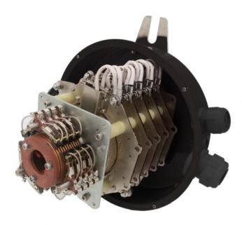
Slip ring collector consisting of power rings coupled with signal rings, designed to transfer electric current from a stationary supply point to a rotating structure, transmitting power and control signals, both analogue and digital.
