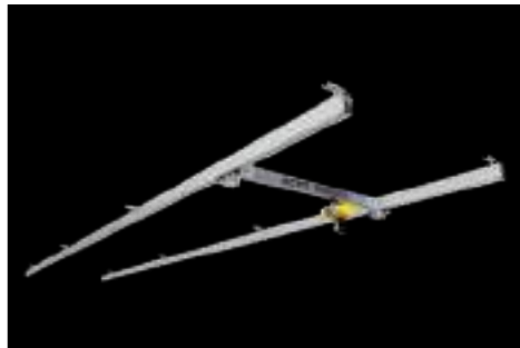
Single girder crane (aluminium bridge and track)
