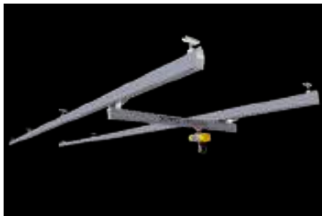
Single girder crane (steel bridge and track)
