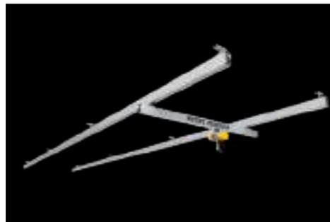
Single girder crane (aluminium bridge and track)
