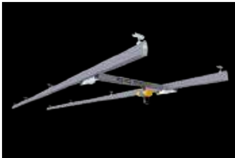
Single girder crane (steel bridge and track)
