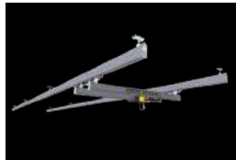
Double girder crane (steel bridge and track)
