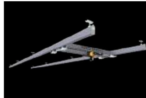
Double girder crane (steel bridge and track)
